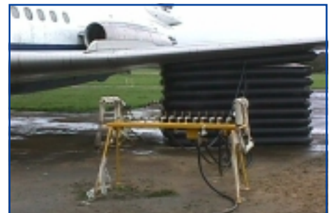
Single Control console and a set of 30 tonne Single Element Airbags.
