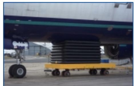
*Nose lift of a DC10 aircraft. 30 tonne Single element airbags were used for the lift, they also acted as a cushion to prevent damage to the aircraft skin.*
